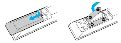
If your remote control does not operate properly, the batteries may need to be replaced. When your remote control is not being used for extended periods of time, remove the batteries to avoid possible damage from battery leakage.
